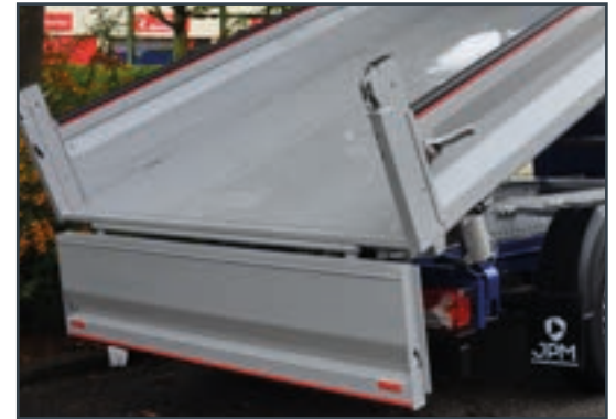
Manual bottom opening door
