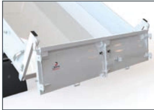
Door with automatic release
