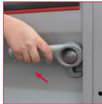
Double safety device and handle incorporated into the sideboard, thus preventing unexpected opening by collision
