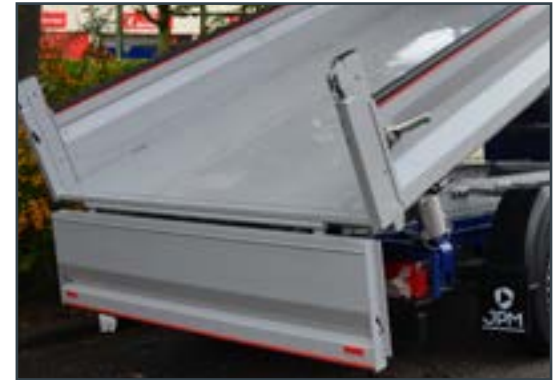
Manual bottom opening door
