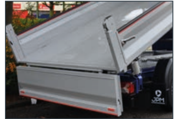
Manual bottom opening door
